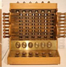
1600s: input data! 1623: first gear-based input-processing calculator by Schickard
