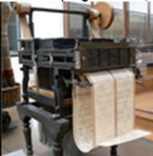
1800: first commercial program-controlled machines (looms) by Jacquard et al. First industrial programmers; software on punchcards
